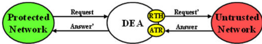
Figure 9-2 Diameter Topology Hiding Trigger Points: Protected-to-Untrusted Transactions
