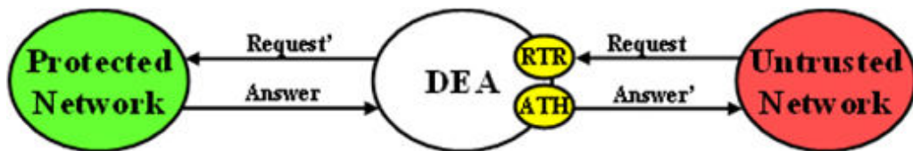
Figure 9-3 Diameter Topology Hiding Trigger Points: Untrusted-to-Protected Transactions
